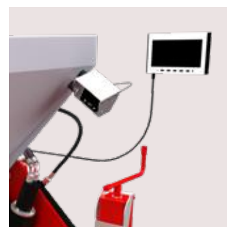
Camera to monitor the filling area.
