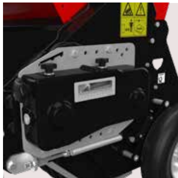
Easy to adjust seed rate gearbox.
