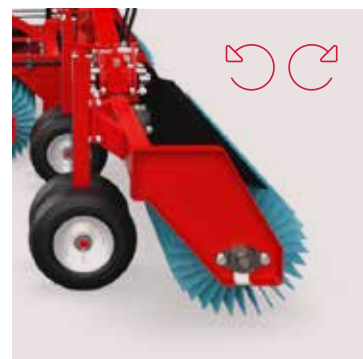
Brushes can be rotated in either direction.
