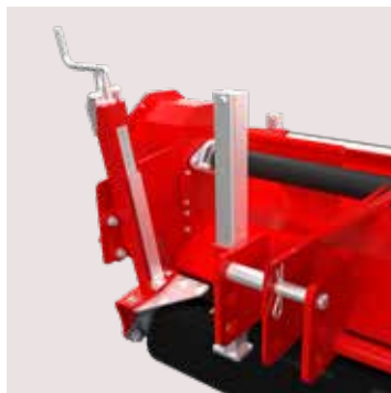
Easy to adjust working depth (1600 & 2000).
