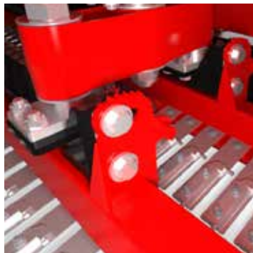
Adjustable tine angle for varying degrees of aggressiveness.
